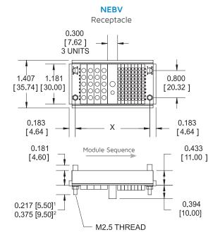
Notes: 1. Standard mounting stud length. 2. For thicker chassis, this longer mounting stud length can be selected by adding the modification code "-479" to the end of the connector part number.
