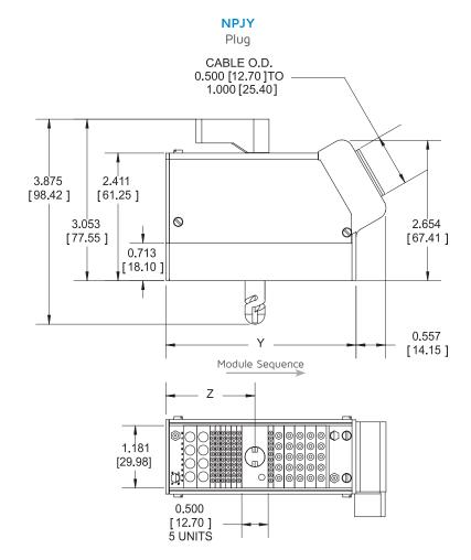
Notes: 1. Frame JY mates with NEBY or NEPJY. 2. Protective dust cover for plug only part number: ZMP0025-XX (XX = number of modules). Dimensions are in inches [mm].
