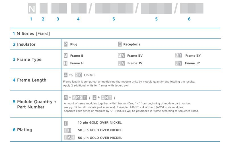
Notes: 1. When part number exceeds 24 characters, please consult factory for special (abbreviated) part number. 2. The plug frame has a built in pin shroud (sockets may be used in plug frames, but not recommended). 3. Consult factory when ordering straight dip solder tails with center jacking version. Special cut out and modification - 872 is required. Dimensions are in inches [mm].
