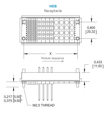
Notes: 1. Standard mounting stud length. 2. For thicker chassis, this longer mounting stud length can be selected by adding the modification code "-479" to the end of the connector part number.
