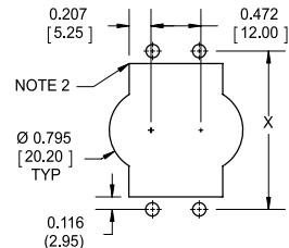
**Notes:** 1. Standard frames are shipped completely assembled with the selected modules mounted. 2. 59.0 oz. in torque for mounting. 3. 0.010 [0.25] maximum radius typical. Dimensions are in inches [mm].
