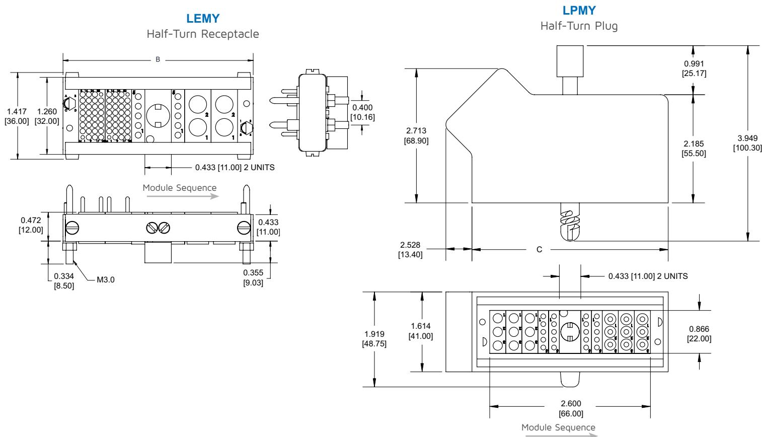
**Notes:** 1. Half-turn plug frame without hood available as LPMY. 2. Allow 2 additional units for frames with Jackscrews
