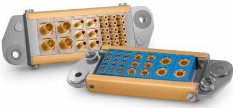
Smiths Interconnect's L Series rugged high density modular connectors employ a do-it-yourself system based on the principle of building blocks. The L Series system is composed of two elements: modules and frames. Modules of various styles and contact types, including signal, power and coaxial, can be combined into custom arrangements within a single connector frame. This allows the user to build a connector that addresses and fulfils their exact requirements with off-the-shelf components.
