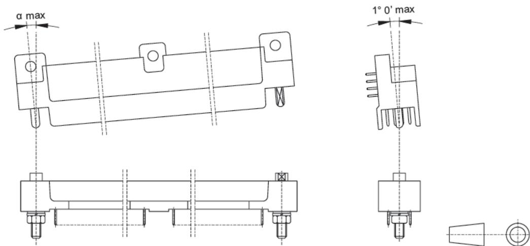
$\alpha = 0^\circ 11'$  for connectors equipped with 220 or 236 contact positions.
