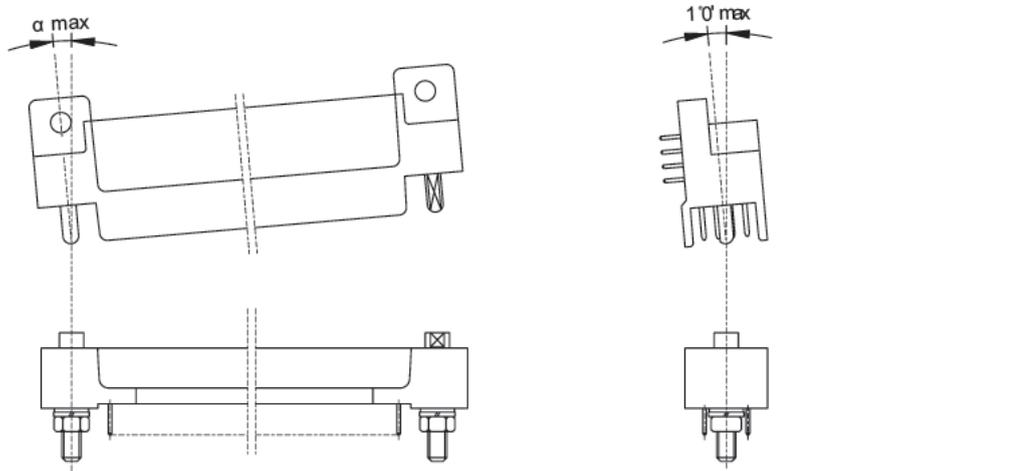
$\alpha = 0^\circ 25'$  for connectors equipped with 42, 82, 110, 126, 158 or 174 contact positions.
